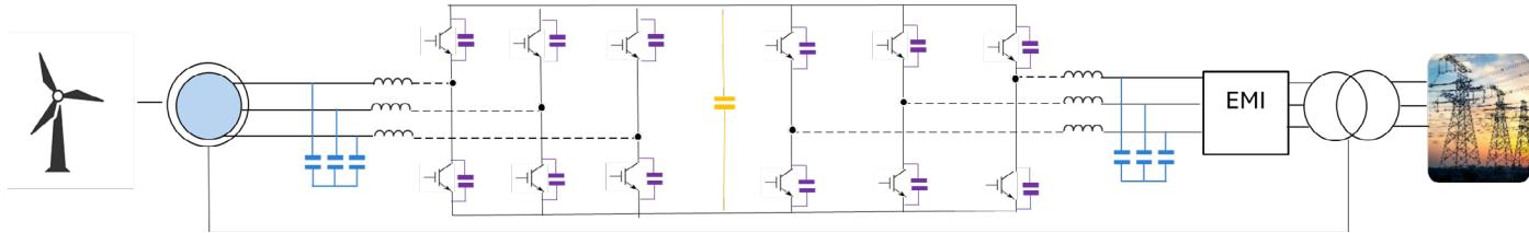
The C44P-T is specifically designed for these situations. Its self-healing properties help protect against electrical overstress. It offers a low-loss profile that limits heat buildup, even under heavy ripple currents. And because it handles high currents with ease, it's ideal for modern converter designs that push power density to the limit.
